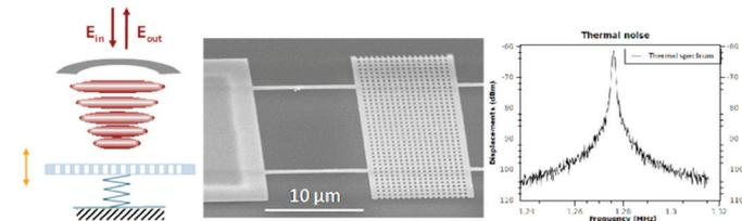
left. Schematics of the optomechanical Fabry-Perot cavity. Center. SEM image of a free-standing InP membrane pierced by a square lattice of holes and acting as mirror at normal incidence. Right. Phase noise spectrum of the reflected field (the peak reflects the Brownian motion of the resonator at room temperature).
