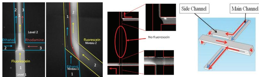
The left panel shows laminar streams co-flowing in 3D different configurations in order to perform multicomponent reactions. The right panel shows the scheme of the "add-and-drop" device and a general view and details of flows in the add-and-drop device : extraction of the 10% of fluorescein flow from the left side of the channel and re-injection on the opposite side. All channels are 100μm wide, 25μm deep.
