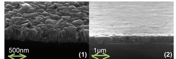
SEM view of a polycrystalline diamond layer (1) before and (2) after the smoothing process
