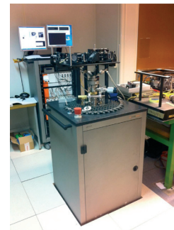
New in-situ lithography machine recently implemented at LPN
