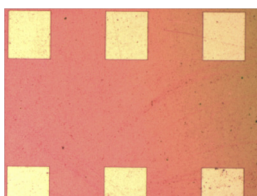
image of Pt pads on PZT thin film (optical microscope)
